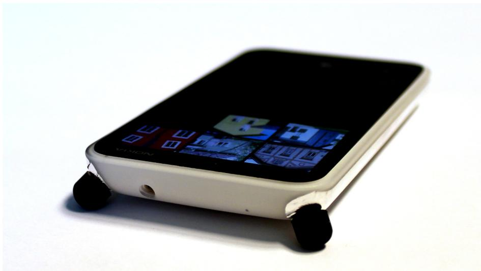
Figure 4.6: Device Touch implementation using capacitive sensing technology. Stylus heads are attached to the corners of the phone and conductive tape is used on the device sides to connect the user’s body to the stylus.
