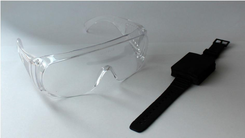
Figure 4.7: Device surrogates used in the study. Smartglasses (left) were simulated with ordinary 3M safety spectacles. Smartwatches (right) were simulated with custom mock-ups built by attaching a Casio watch band to a small block of polystyrene foam.
