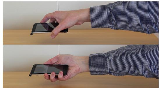
Figure 7. Different grips for Device Touch: a) from above (top), and b) from below (bottom).
