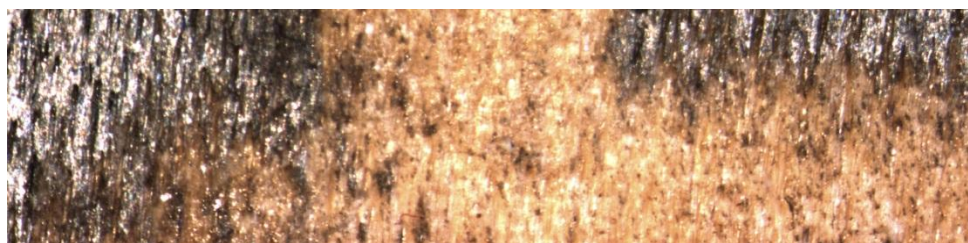
Figure 15 A microscope image of silver NP ink on plywood substrate. The grains on the plywood are in the vertical direction in the image.
