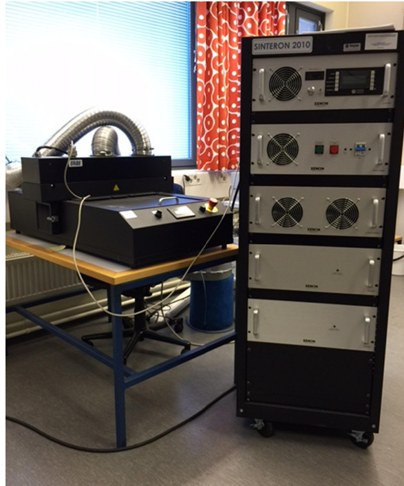
Figure 18 Xenon Sinteron 2010-L system which is used in this study.
