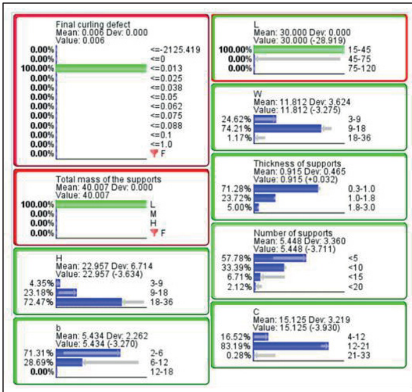
Figure 59. Backward simulation to minimize curling defect and supports' mass for small-sized parts (15 < L < 45)
