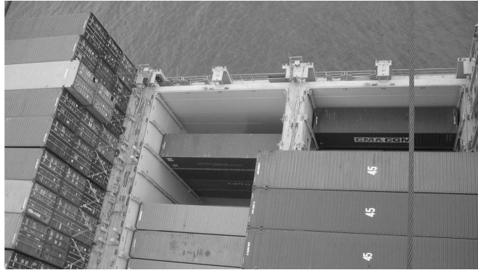
Figure 9.1 The ship hold and vertical cell guide bars for containers. Snag load may occur when a container is jammed into guide bars during lifting (Konecranes Plc).
