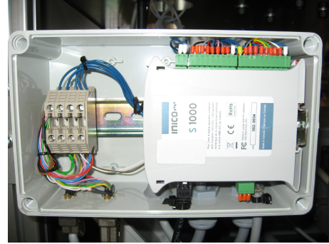
(b) A production device can be viewed as a web service when it is connected to an appropriately programmed controller.
