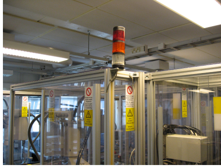
(a) The light tower web service represents a type of signal tower device used in production systems.
