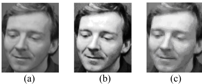
Figure 17: The examples of luminance adjustment: (a) Original image, (b) After histogram equalization, (c) After DC Normalization.
