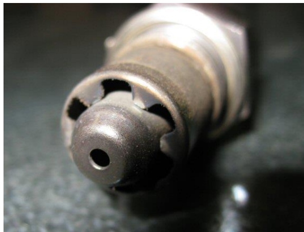
Figure 7. A Bosh LSU 4.0, wideband, planar type, lambda sensor after a challenging trial run with a 20 kW pellet boiler.
