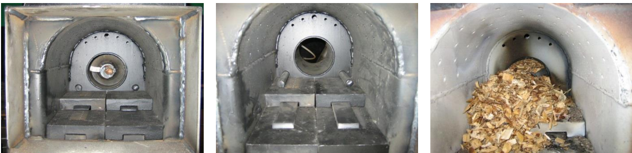
Figure 10. The 80 kW wood chip burner. Primary air feeds upward from the grate. Secondary air is fed from the walls and ceiling. The grate sweepers are at the innermost (left) and outermost (middle) positions. Typical fuel pile on the grate (right). (Korpela, 2006).
