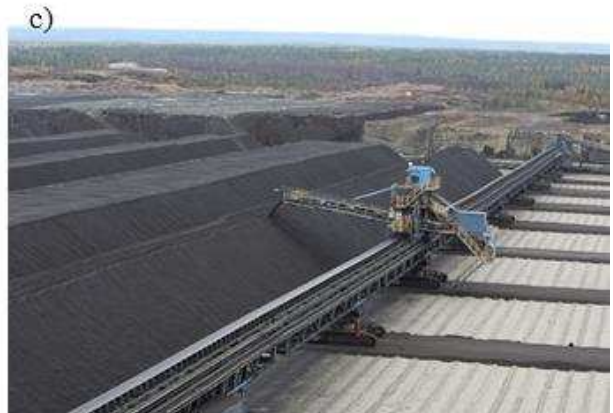
Figure 8. a) Schematic diagram of the Talvivaara process from mining to metal recovery. b) Photograph of the mine site. c) Heap stacking. Photos: Marja Riekkola-Vanhanen.
