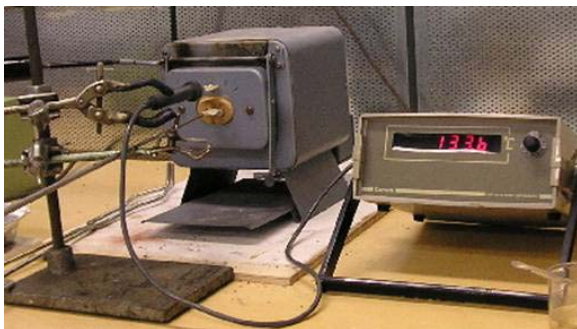
Figure 4.11. ISO 562 test equipment at TUT.
