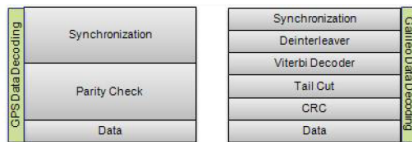
Figure 8. Data decoding process for GPS and Galileo
