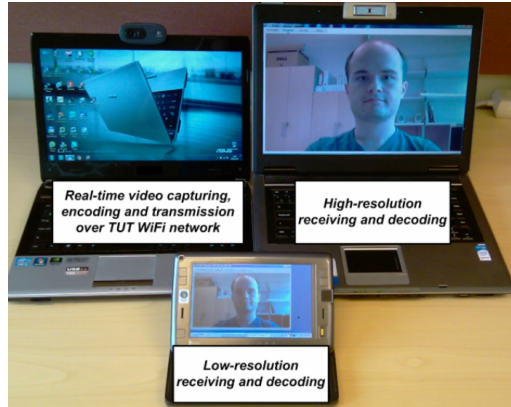
FIGURE 4.10: Illustration of scalable video transmission over wireless network of Tampere University of Technology (TUT) based on the proposed 3-D DWT codec
