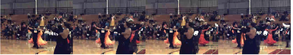
Fig. 5: x.264 ultrafast mode, Bit rate = 2000 kbps, Y-PSNR=26.422, Encoding speed = 10.6 fps
