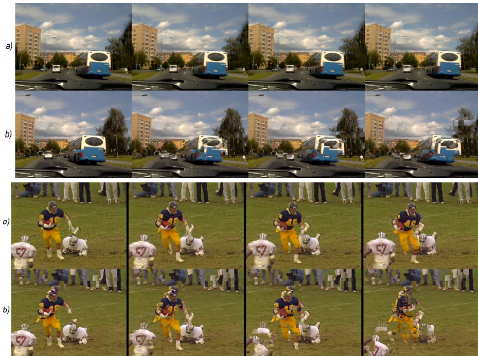
FIGURE 4.4: Visual comparison for 5% packet loss. a) Proposed 3-D DWT b) H.264/SVC (JSVM 9.8)
