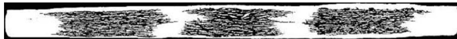
Figure 6.2: Cross-section of a 60-filament Bi-2223/Ag tape of thickness 0.235 mm and width 4.05 mm.
