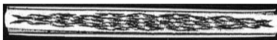
Figure 5.1: Cross-section of a 55-filament Bi-2223/Ag HTS tape specimen made by American Superconductor.
