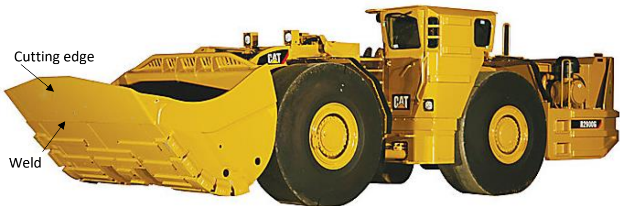
Figure 5.15. CAT R2900G underground mining load-haul-dump loader [119].
