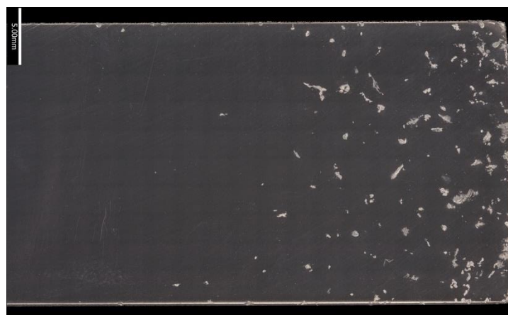
Figure 6.2. Optical profilometer image of a polished 400HB steel sample tested for two seconds with the impeller-tumbler. Scale bar is 5 mm.
