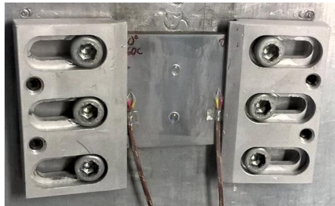
Figure 5.12. Two impact marks on the steel plate sample attached to the sample holder.
