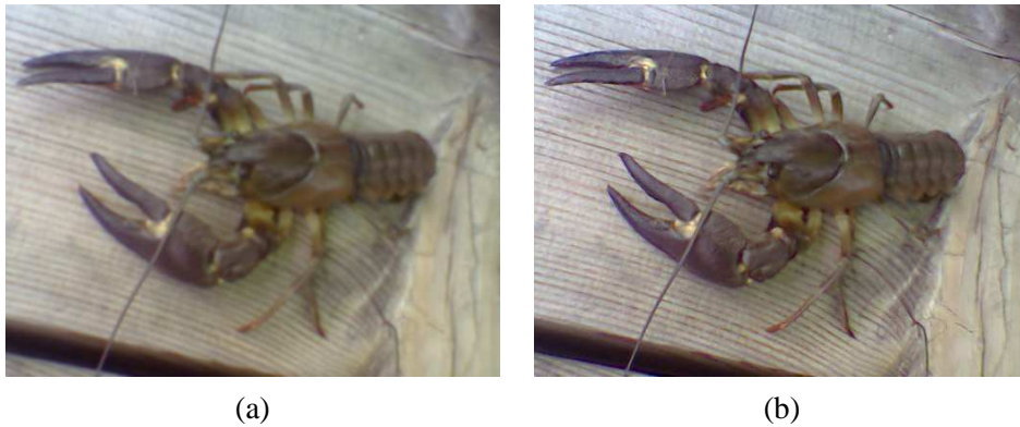
Figure 3.8: (a) Test image taken with a Nokia-6600 camera phone and reconstructed with the default processing chain. (b) Final image processed with the proposed deblurring of the raw data after 4 iterations, and reconstructed with the same chain.
