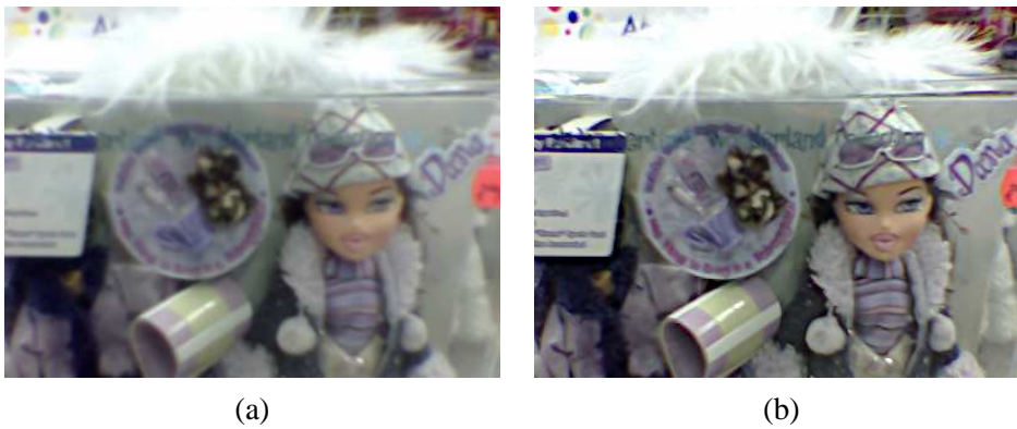
Figure 3.9: (a) Test image taken with a Nokia-6600 camera phone and reconstructed with the default processing chain. (b) Final image processed with the proposed deblurring of the raw data after 3 iterations, and reconstructed with the same chain.
