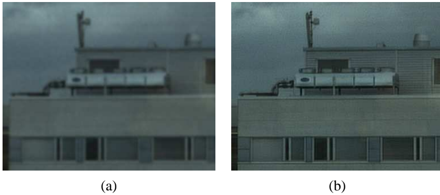
Figure 2.11: Example results using input sequence from digital camera (Micron board MI-SOC1310). 6 cropped frames from an uncompressed video sequence are used. (a) Reference frame zoomed by 2 using bicubic interpolation. (b) Super-resolution result using MAP technique, 5 iterations.
