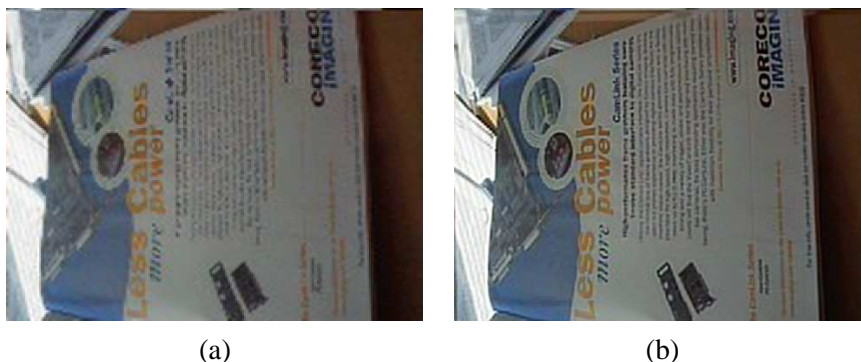
Figure 2.10: Example results using input sequence from a digital camera. 16 JPEG compressed images are used. (a) Reference frame zoomed by 3 using bicubic interpolation. (b) Super-resolution result using iterated back-projection technique, 1 iteration, real time operation.
