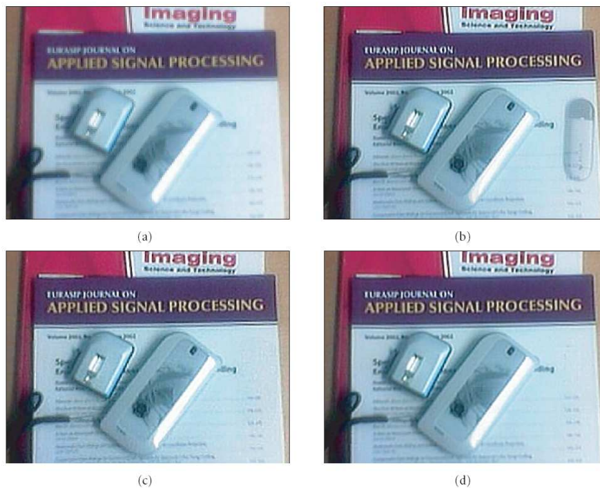
Figure 6.12: The super resolved images using the proposed algorithm. 5 LR images were cropped from VGA images taken with a cameraphone (Nokia 9500). One outlier object appears in the last frame. (a) Zero order interpolated reference frame, zoom factor 2; (b) result using mean fusing, (c) result using median fusing, and (d) super-resolved image using the proposed method.
