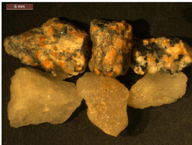
Fig. 2. Stereomicroscope image of Sorila granite (upper) and Haluna quartz particles.
