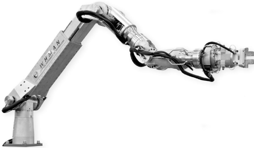
Figure 22: The Water Hydraulic Manipulator for ITER Divertor maintenance, developed by Tampere University of Technology's Department of Intelligent Hydraulics and Automation
