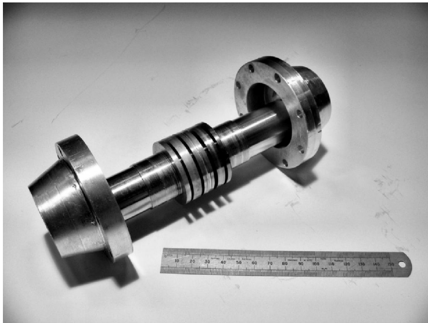
Figure 62: Load segregated joint
