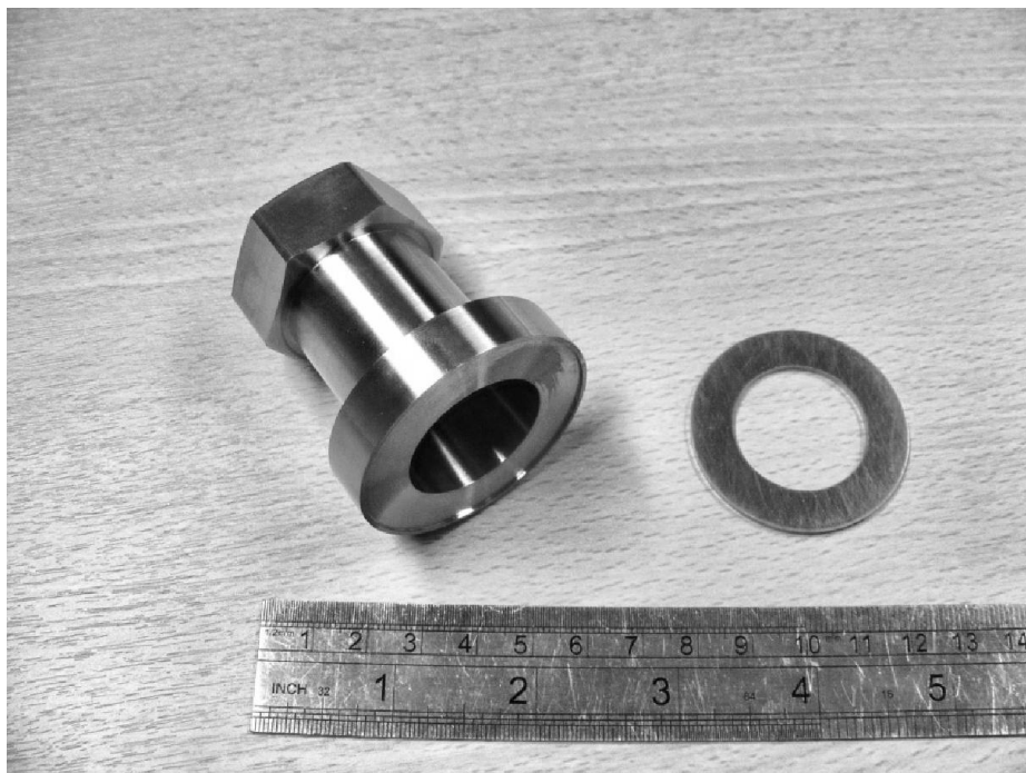
Figure 57: Pilot study pipe joint – Stainless Steel body (left) and Ni interface washer (right)
