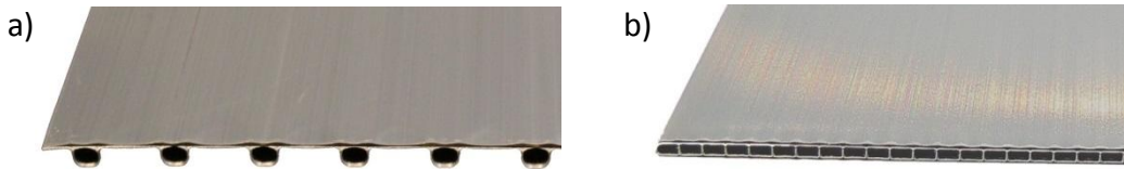
Figure 9. Extruded aluminium profiles: a) a profile with circular fluid channels behind the planar plate, and b) planar profile with rectangular fluid channels inside the shape.
