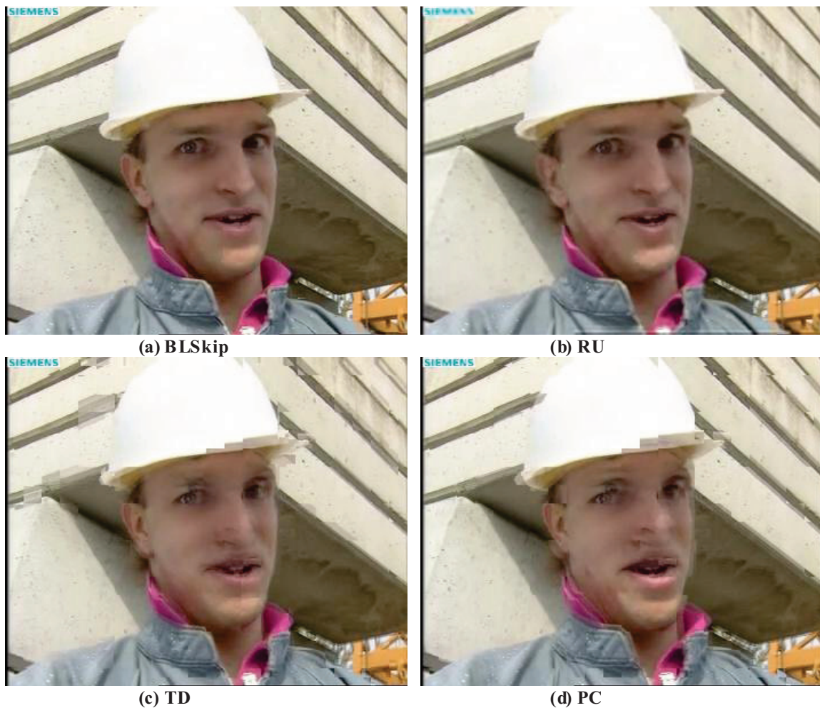
Fig. 21: Subjective quality comparison of concealed pictures for foreman packet loss rates of base layer and enhancement layer are both 3% and QP=28.
