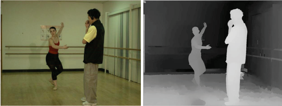
Fig. 32: A texture video frame and its associated depth map.
