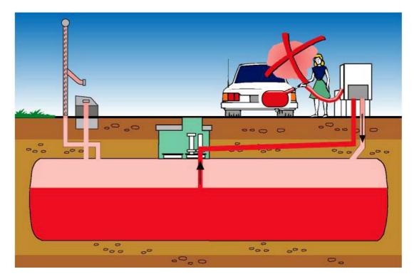
Fig. 1.8. Illustration of vapour recovery stage 2-system.
