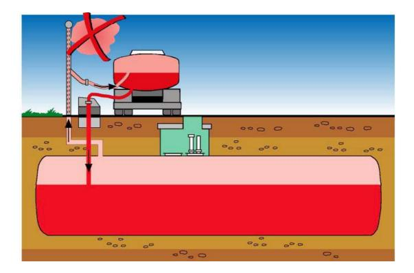
Fig. 1.7. The scheme of vapour recovery stage 1-system.
