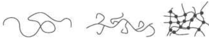
Figure 1.3: Chain structure of polymers: linear chain, branched chain and cross-linked network. The molecules are connected through chemical bonds.
