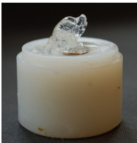
Fig. 4 Gelled cellulose solution from 100 % AHP pulp on top of spinneret
