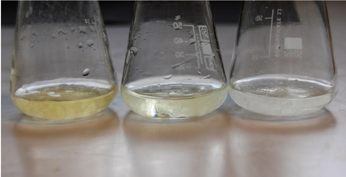
FIGURE 18 Reaction of fibres with bromine. Samples from left to right: reference fibres, 10/90-mixture fibres and 25/75-mixture fibres.
