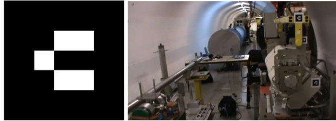
Figure 3: Left image shows an example of a binary-based marker. Right image shows the real device to maintain (i.e. the collimator) with the attached markers.
