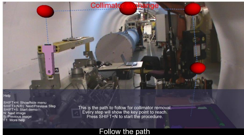
Figure 7: Instructions showing the path to follow for the collimator removal. This step is displayed after the hook-spreader alignment and before the actual collimator removal. When the operator press the right key, the first key point starts to flash, showing the order to follow.
