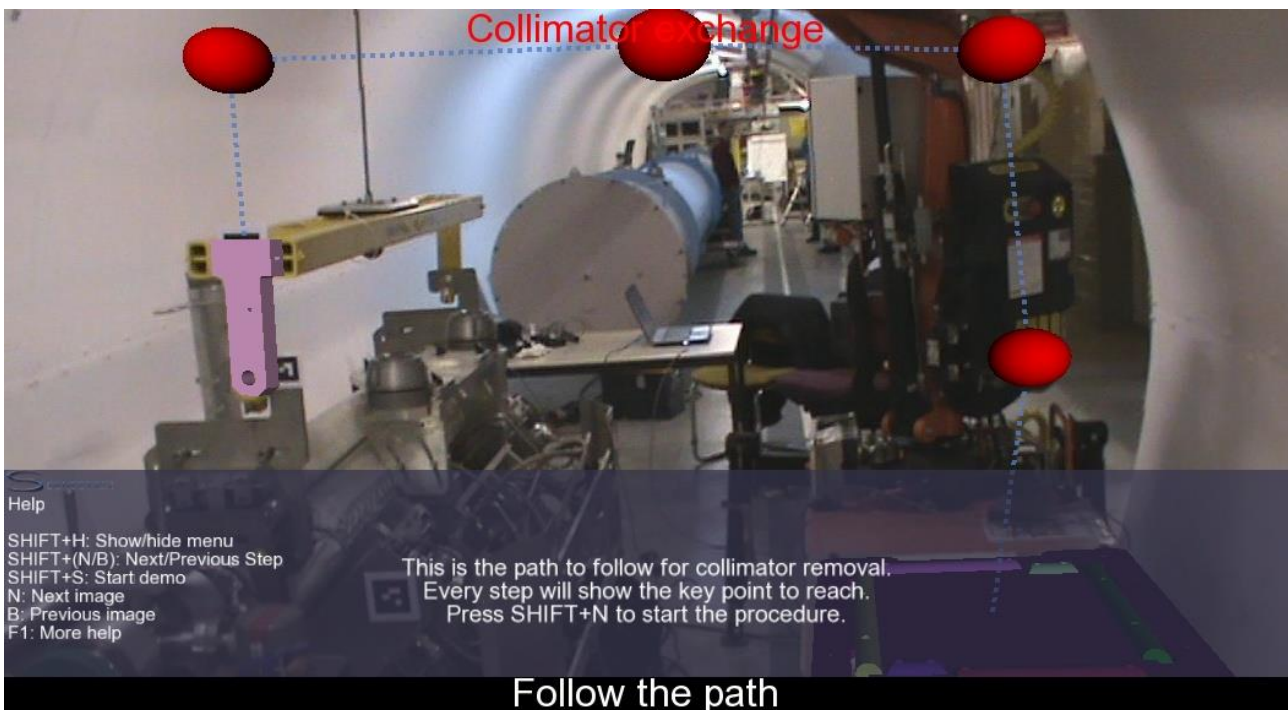
Figure 9. Example of a maintenance application using the developed AR engine. The image shows a prototype for aiding collimator exchange at CERN. The image and the related prototype details can be found in Publication VI.
