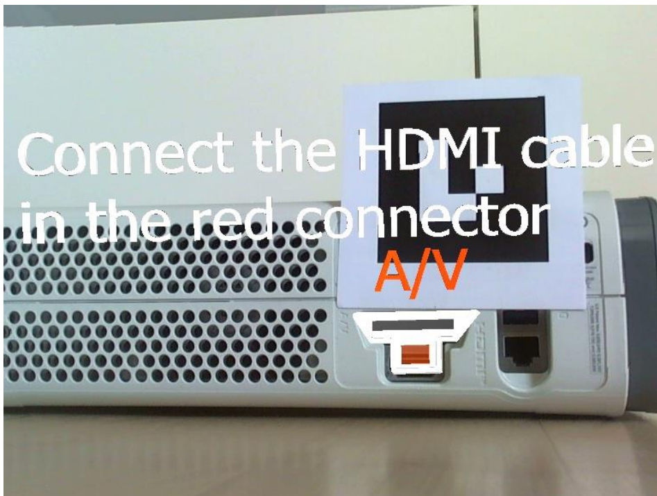
Figure 2. Example of a computer vision-based AR application. The marker visible in the image is recognised by computer vision algorithms, and it is used as the origin for the positioning of the virtual elements in the final scene. In this particular example, the application guides the user to connect the cables to the device. The text and 3D model explain the appropriated connector to use for the current step.
