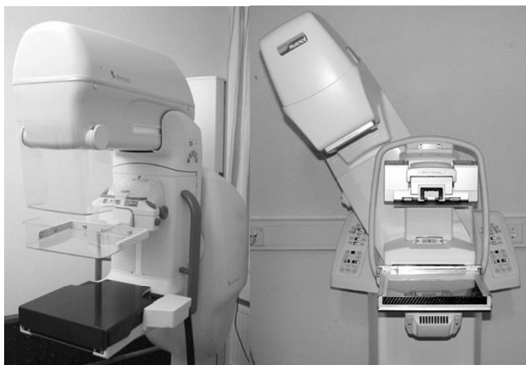
Figure 17. The prototypes of full field digital breast tomosynthesis system, Diamond DX and Nuance based on a -Se FPD technology.
