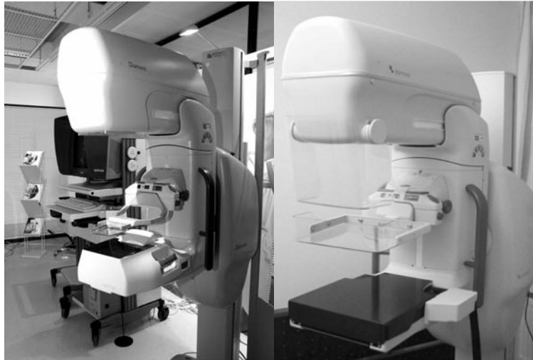
Figure 8. On the left side Diamond Delta 32 for diagnostic breast tomosynthesis system. This system incorporates a CCD small-area detector with 48\ \mu\text{m} pixel size, and is using TACT 3D technology. On the right side the prototype of tomosynthesis FFDM system (Diamond DX) based on \alpha -Se technology with 85\ \mu\text{m} pixel size.
