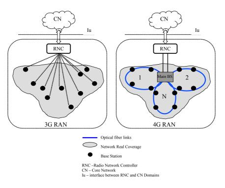
Figure 9. The models of RAN configuration
