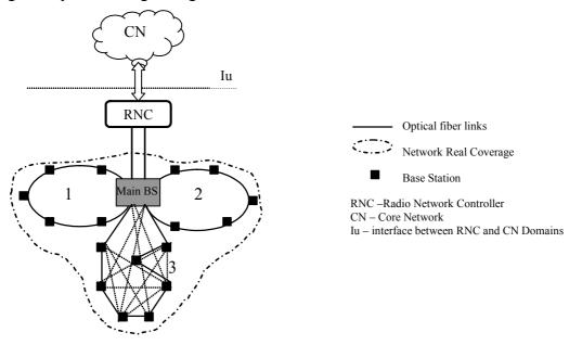
*Figure 12.* An example of the 4G-RAN ring configuration
