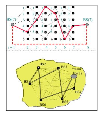
*Figure 13.* An example of the determination of the ring configuration with the minimum cost for 7 BSs in 4G RAN
