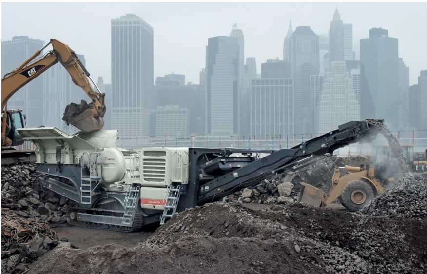
Figure 5. A typical product of the case company. LT106 Lokotrack is a mobile rock crushing unit. Source: Metso MAC
