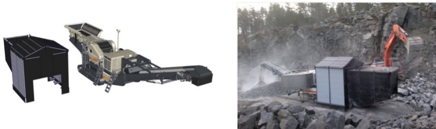
Figure 39. Virtual prototyping was utilized in a rock crusher noise reduction concept development. On the left is a digital model of the concept, and on the right side is the physical prototype in the field test. The assembly and functionality of the noise reduction module was assessed with virtual prototyping. (Source: Metso MAC.)
