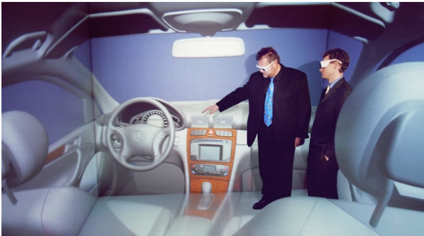
Figure 1. Utilizing virtual prototyping and virtual environments in designing and evaluating user interfaces of a passenger car (source: Mercedes Benz).
