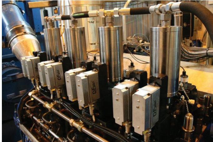
Picture 2 EHVA on the 4-cylinder W20 engine
