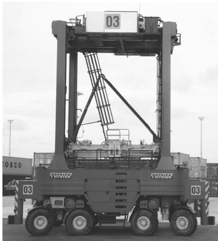
Figure 2. An automated straddle carrier, AutoStrad. [28]
