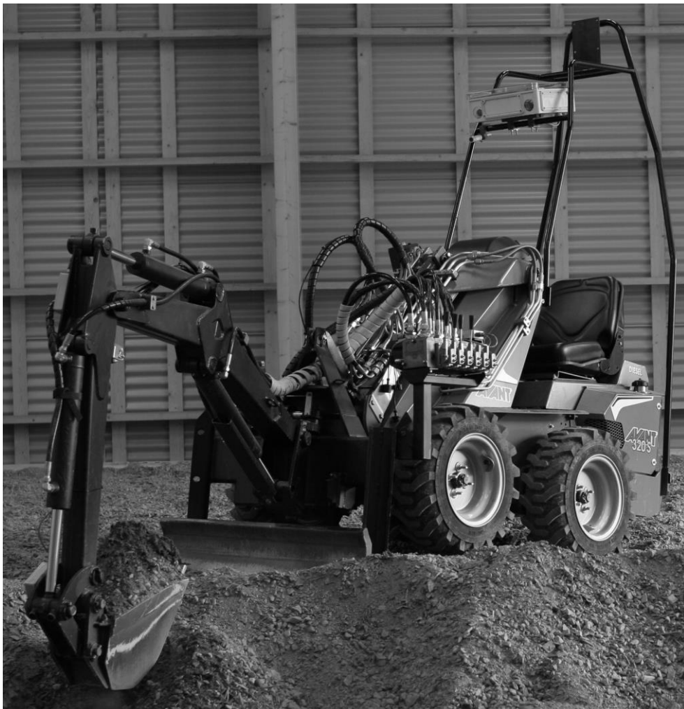
Figure 28. Modified wheel loader with excavator attachment.
