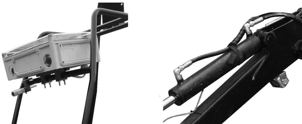
Figure 31. Cameras on wheel loader and excavator stick boom.
