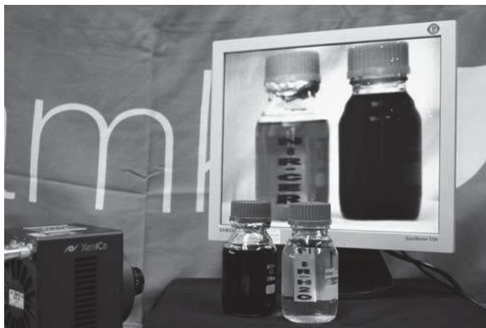
FIGURE 7.18 Near-infrared imaging used in moisture detection and in seeing through a kerosene-based liquid.
