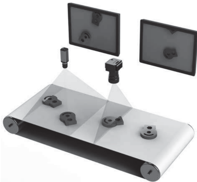
FIGURE 7.4 Matrix camera (on the left) images in two dimensions and line camera (on the right) images one line at a time, and computer combines the lines as a continuous 2D image, as seen on the right.
