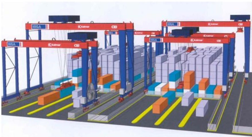
Figure 35. A 3D illustration of the ASC block (Cargotec). Figure used with permission from Cargotec.
