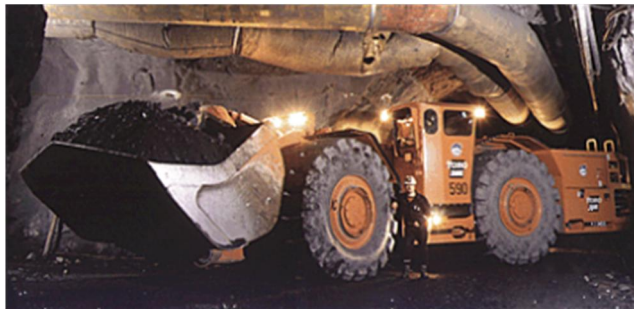
Figure 21. An electrically powered LHD in the Kiruna mine (Sandvik). Reprinted with permission from Sandvik Mining and Construction.
