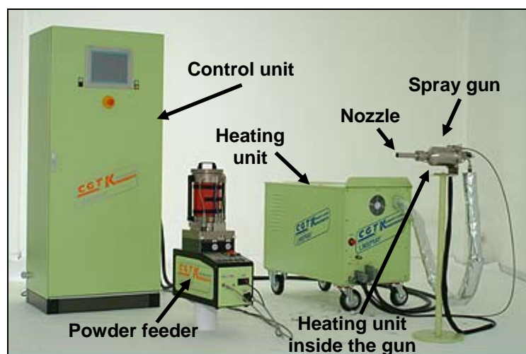
Figure 30. Cold Gas Technology GmbH (CGT) Kinetiks 4000 high-pressure cold spray system [136].
