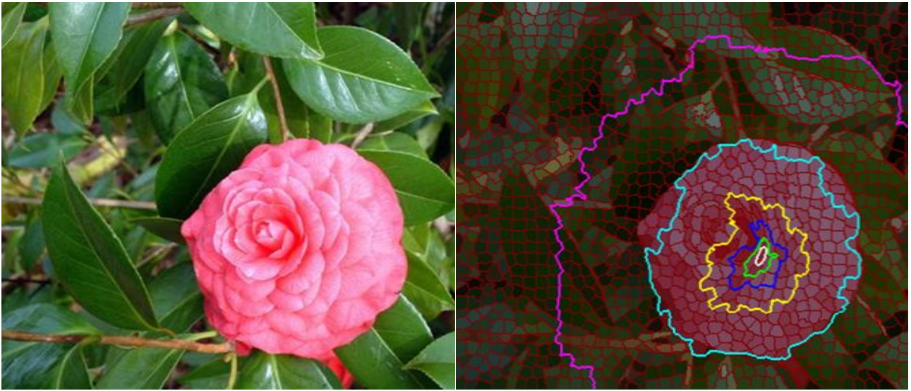
Figure 14 An image from MSRA1000 dataset, boundaries of a superpixel, its 1 st , 2 nd , 3 rd , 4 th and 5 th neighbor sets shown in white, blue, yellow, cyan and magenta colors respectively. Other superpixel boundaries are shown in dark red color.
