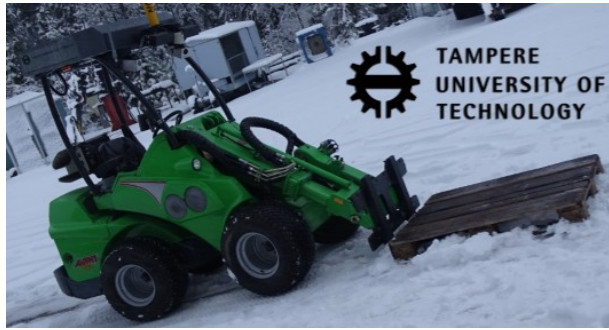
Figure 1.2: Avant autonomous forklift; AUT's mobile laboratory
