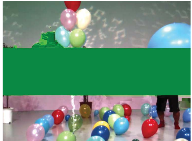
Figure 9. When using P- and B-frames motion vectors pointing out from the undecoded region (middle slice) propagate bogus colors into the slices which we intend to decode.
