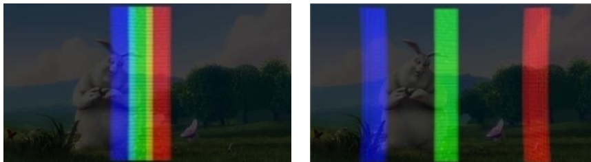
Figure 30. Left: Adjacent rendering nodes consume adjacent, slightly overlapping parts of a source view. Red, green and blue overlays represent the areas of the image used by three rendering nodes that drive adjacent projection modules. Right: Rendering nodes that drive projection modules positioned further away from each other use a disjoint set of pixels from the same source view.
