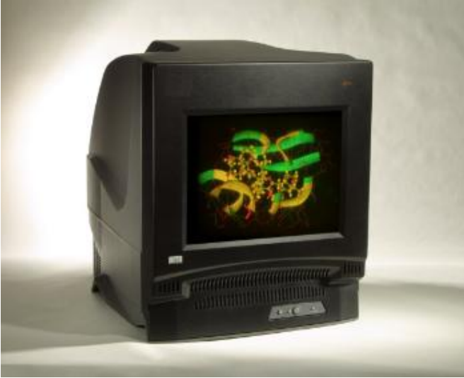
Fig. 12 DepthCube volumetric display. Image courtesy of LightSpace Technologies Inc. [provisional permission to be finalized]
