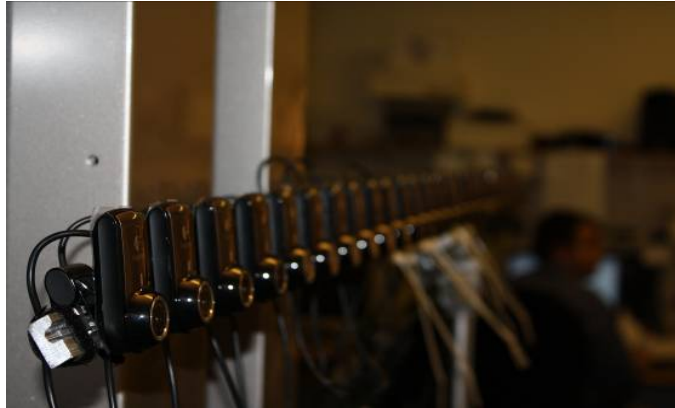
Figure 3. Camera array consisting of 27 CCD USB cameras. Together they capture up to 18MPixels.
