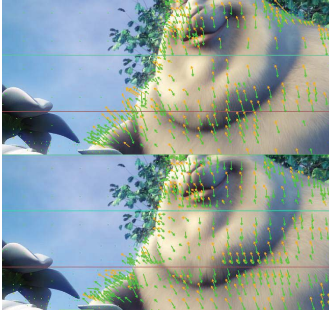
Figure 10. Difference of motion vectors in normal encoding and with self-contained slices. Notice that in the normal case (top) motion vectors cross slice / tile boundaries. In the self-contained case (bottom) no motion vectors cross the slice / tile boundaries.
