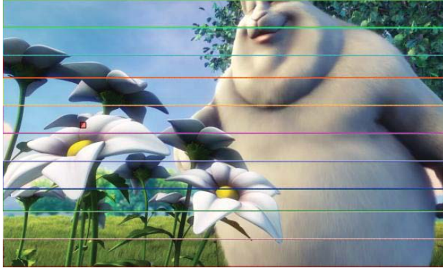
Figure 6. A frame subdivided into horizontal H.264 slices. In an I-frame, these slices can be decoded independently.
