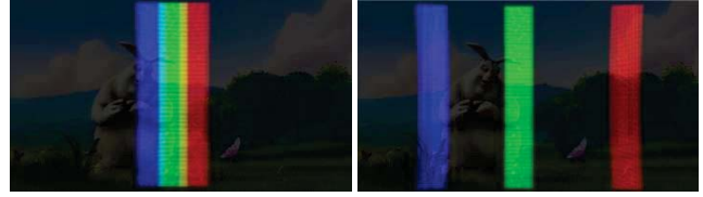
Figure 3. Left: Adjacent rendering nodes consume adjacent, slightly overlapping parts of a source view. Red, green and blue overlays represent the areas of the image used by three rendering nodes that drive adjacent optical modules. Right: Rendering nodes that drive optical modules positioned further away from each other use a disjoint set of pixels from the same source view.
