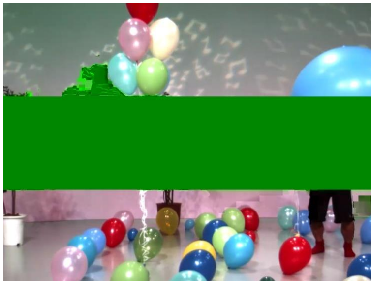
Figure 33. When motion vectors point out from the undecoded region (middle slice), they propagate bogus colors from the undecoded region into the slices which we intend to decode
