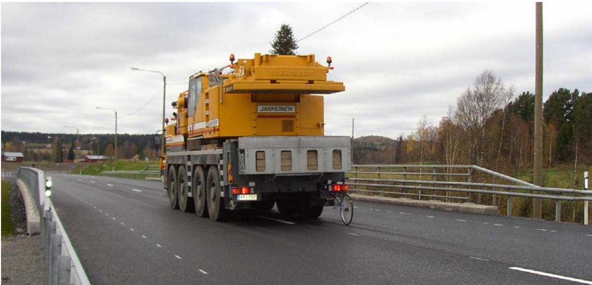
Figure 4.7. The mobile crane equipped with a speed measuring wheel during the braking test at Haavistonjoki Bridge. Mobile crane: Liebherr LTM 1090, dead weight 56 tonnes.
