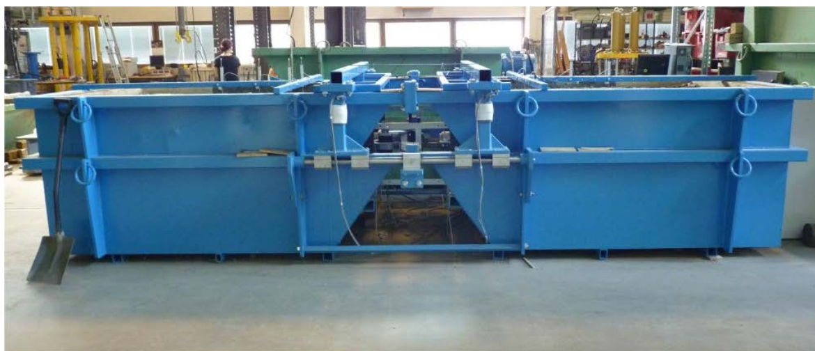
Figure 8.3. Loading device called the “Integral bridge simulator”.
