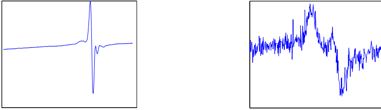
Figure 5.5: A typical PSF of the FGS instrument(left), and an observation of the asteroid Kleopatra with the FGS(right).
