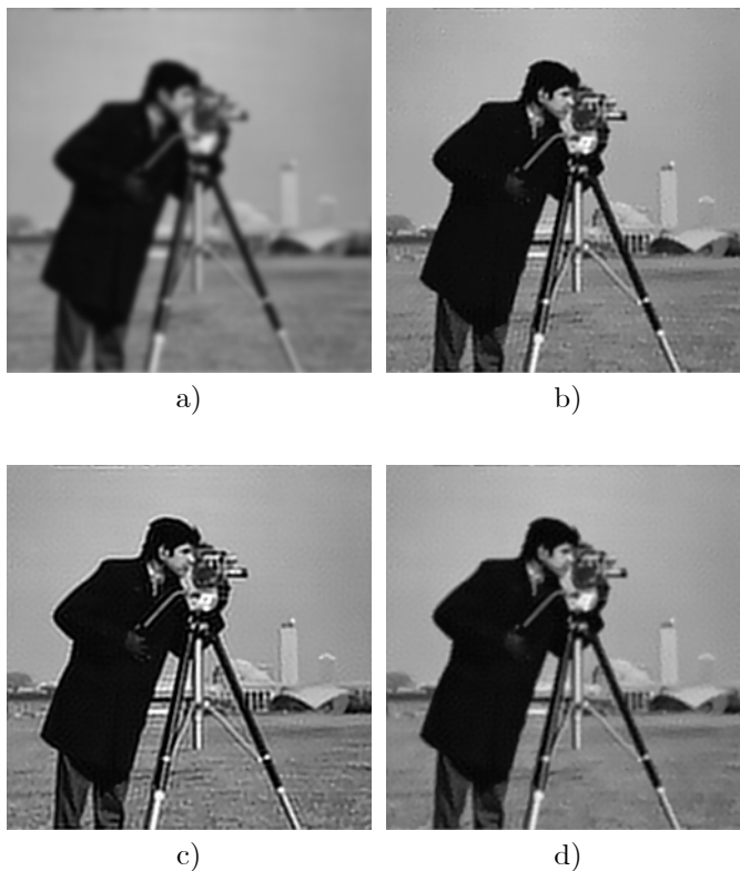
Figure 4.16: Experiments for Cameraman test image: a) noisy blurred image with Gaussian PSF \sigma_{blur} = 2 ; b) reconstructed using the regularization technique (Katkovnik, 2005) after the blur and its parameter has been identified as Gaussian PSF with \sigma_{blur} = 2 (ISNR=3.88 dB); c) the original image was blurred by the Gaussian PSF with \sigma_{blur} = 1.835 and then reconstructed using the regularization technique (Katkovnik, 2005) after the blur and its parameter has been identified as Gaussian PSF with \sigma_{blur} = 2 (ISNR=3.20 dB); d) the original Cameraman image was blurred by Gaussian PSF with \sigma_{blur} = 2.165 (This blurred image does not differ visually from the one in (a)) and then reconstructed using the regularization technique (Katkovnik, 2005) after the blur and its parameter has been identified as Gaussian PSF with \sigma_{blur} = 2 (ISNR=3.22 dB).
