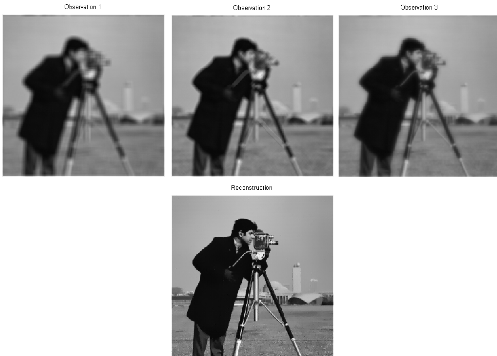
Figure 4.7: Illustration of Cameraman image restoration (lower row) from its three blurred noisy observations (upper row).
