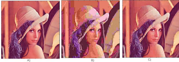
Figure 3.19: Compression results. Original scene (A), Conventional (bilinear+JPEG) CR=125, PSNR=23dB (B) Alternative (JPEG+bilinear) CR= 125, PSNR=30,8 dB.
