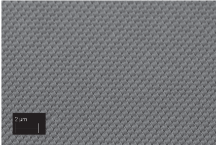
FIGURE 1. SEM picture of the moth eye surface pattern.
