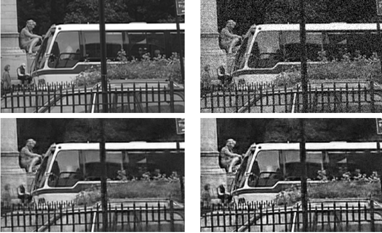
Figure 4.5. Top row: noise-free (left) and noisy (right) frame of the sequence Bus having intensity range of [0,255] corrupted by i.i.d. additive white Gaussian noise with standard deviation \sigma = 25 . Bottom row: sharpening results of V-BM4D using \alpha = 1.1 (left) and \alpha = 1.25 (right).
