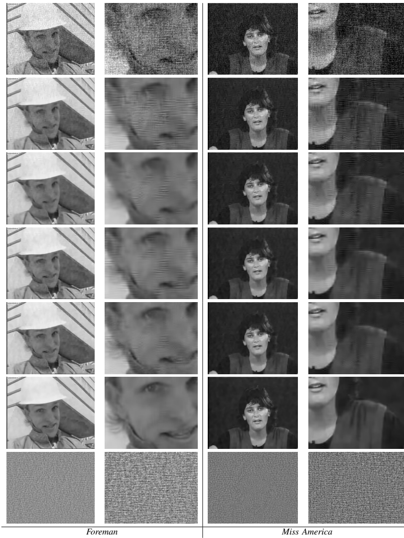
Fig. 11. From top to bottom: denoising results of WR, CR, WRWF, RF3D, E-RF3D, and the FP estimate obtained from E-RF3D for Foreman and Miss America corrupted by synthetic noise having \varsigma_{\text{RND}} = \varsigma_{\text{FPN}} = 15 .
