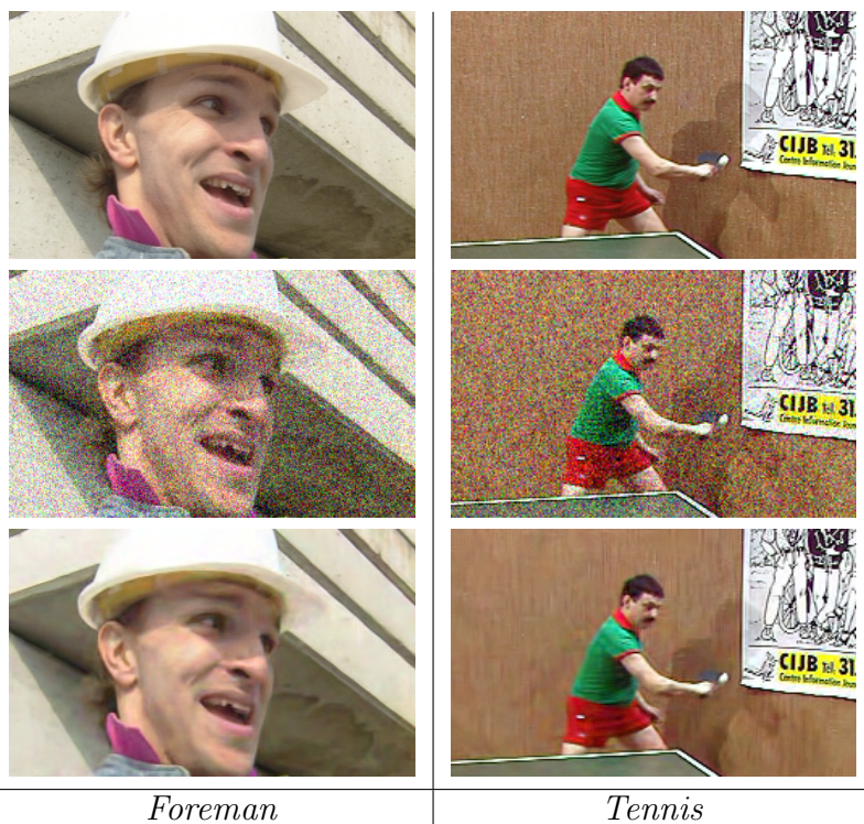
Figure 4.3. From top to bottom: noise-free frame, noisy frame, and V-BM4D denoising results for the grayscale and color sequence Foreman and Tennis . The sequences have intensity range of [0,255] and are corrupted by i.i.d. additive white Gaussian noise with standard deviation \sigma = 40 .
