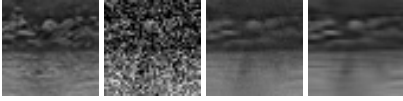
Fig. 3. V-BM4D two stage denoising of the sequence Coastguard . From left to right: original video y , noisy video z ( \sigma = 40 ), result of the first stage y^{\text{ht}} (frame PSNR 28.58 dB) and final estimate y^{\text{wic}} (frame PSNR 29.38 dB).
