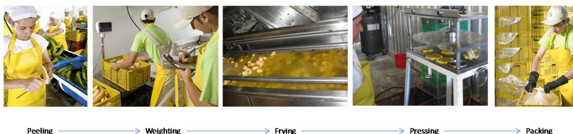
Figure 23. Process of making plantain ripened patacones 49
