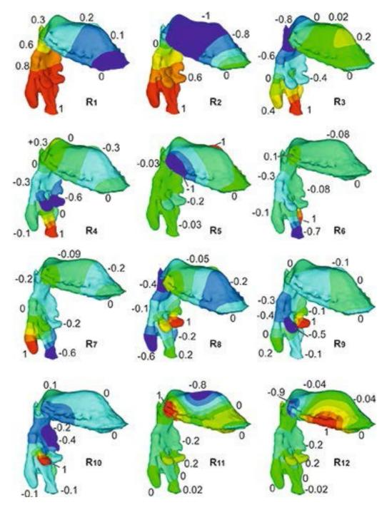
Figure 9. Computed acoustic mode shapes of vibrations for resonance frequencies  $R_1$ - $R_{12}$  of the vocal tract FE model for vowel [a:]. The pressure amplitudes are normalized for maximal values in each mode.
