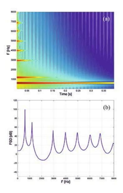
Figure 7. Numerically simulated spectrogram of the acoustic pressure computed at 10 cm in front of the mouth (upper panel) and the power spectral density of the response (lower panel) excited by a short airflow velocity pulse at the vocal folds using the simplified "1D" symmetric model of the vocal tract shown in figure 3c.
