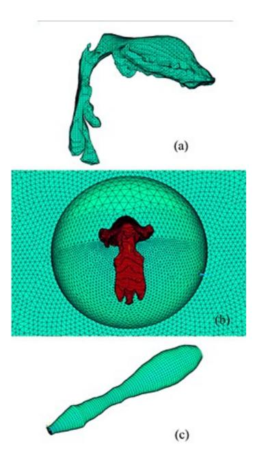
Figure 3. FE models of the vocal tract for the vowel [a:]: a) 3D model constructed from the CT images, b) full 3D model including the surrounding infinite acoustic space used for simulation of sound propagation from the mouth, c) simplified fully symmetric model constructed from the volume model using the cross-sectional areas of measured along the vocal tract from the vocal folds to the lips.
