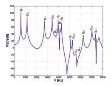
Figure 6. Power spectral density of the acoustic pressure computed at the distance of 10 cm in front of the mouth excited by a short airflow velocity pulse at the vocal folds using the full 3D model of the vocal tract shown in figure 3b.
