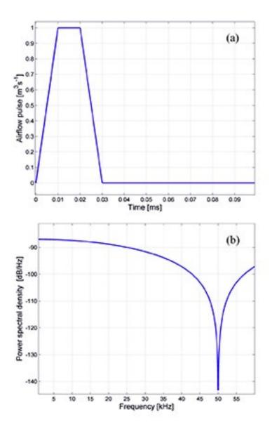
Figure 4. Airflow velocity pulse used for the excitation of the FE model: a) in the time domain, b) in the frequency domain.
