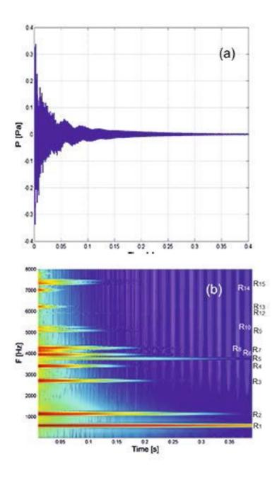
Figure 5. Transient response in time domain of the acoustic pressure computed at the distance of 10 cm in front of the mouth excited by a short airflow velocity pulse at the vocal folds (upper panel) and numerically simulated spectrogram of the sound signal (lower panel) using the full 3D model of the vocal tract shown in figure 3b.
