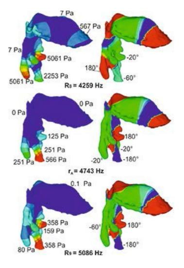
Figure 10. Absolute values of the acoustic pressure inside the vocal tract (left) and the corresponding phase shifts (right) between the excitation harmonic signal and the response for the resonance frequencies  $R_8$ ,  $R_9$  and at the main antiresonance  $r_A$ = 4743 Hz in between.
