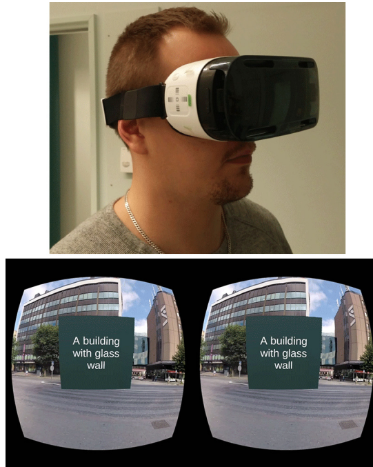
Fig. 2. Top: Amaze360 physical setup. Bottom: Amaze360 application view. The video is shown as a stereoscopic presentation. Activated hotspot is shown at the center of screen.
