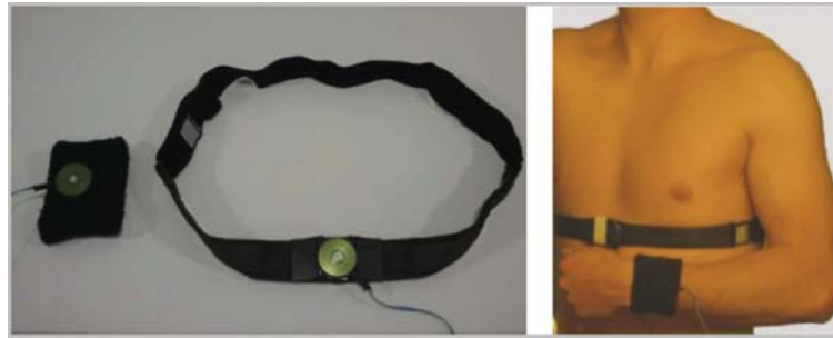
Fig. 1. Attachment of C2 actuators inside a wristband and a chest strap (left), and their locations in a body (right). Pictures of the chest strap with permission of Polar Electro Oy.
