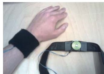
Figure 1. Wrist actuator attached under a wristband and backside view of chest actuator attachment to a chest belt.
