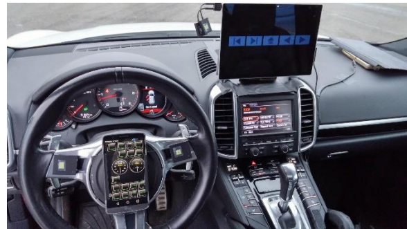
Fig. 6. Placement of the AEE unit and Microsoft Surface Pro device in the test vehicle.
