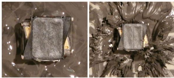
Fig. 2. Active / Passive Actuation Engine with Lofelt L5 actuators (left) Mediation Enabled: MRF in fluid State, (right) Mediation Disabled: MRF in solid State.
