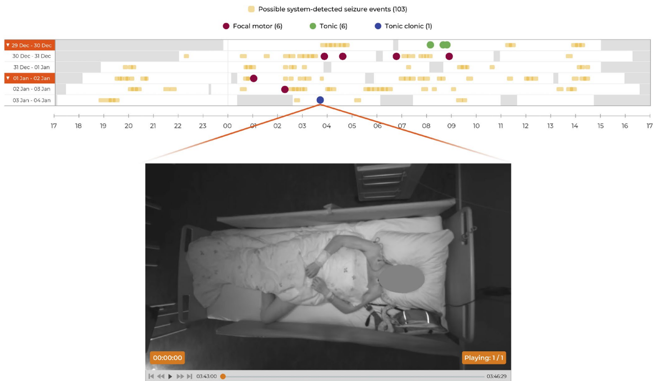
FIGURE 3 Graphical user interface view. Epochs detected by the algorithm (seizure candidate events) are depicted over a 6-day period with a lighter color and small squares. Three different types of seizures were identified by human annotators and marked by larger dots. The time of the day is represented on the x-axis. White background color refers to registration periods. The videos of the epoch can be reviewed by clicking on a dot (subwindow)
