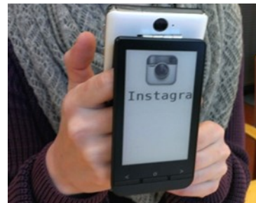
Figure 1. Illustration of the prototype. A hinge enables the user to hold the phone without covering the display with their fingers.
