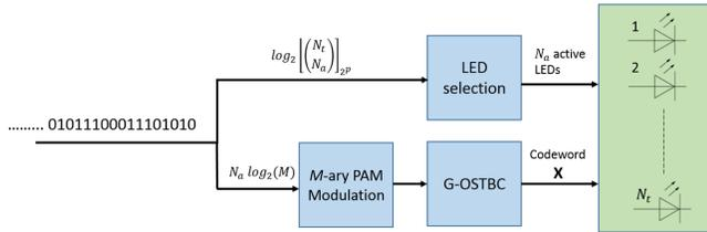
Fig. 1. Generalized STBC-MASM transmitter
