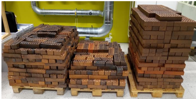
Fig. 1. Two left pallets filled with 3rd class tiles, right side pallet stacked with 2nd class tiles (9 lower rows) and 1st class tiles on top.
