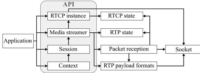
Fig. 2. Software architecture of uvgRTP.
