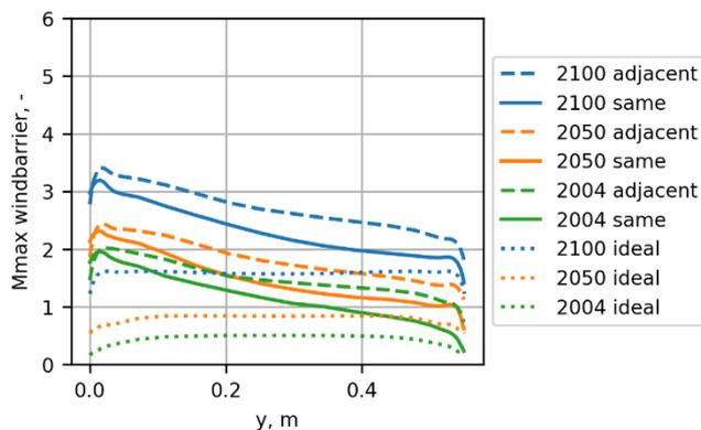
**Figure 3.** Maximum mould index at the interior surface of wind barrier.
