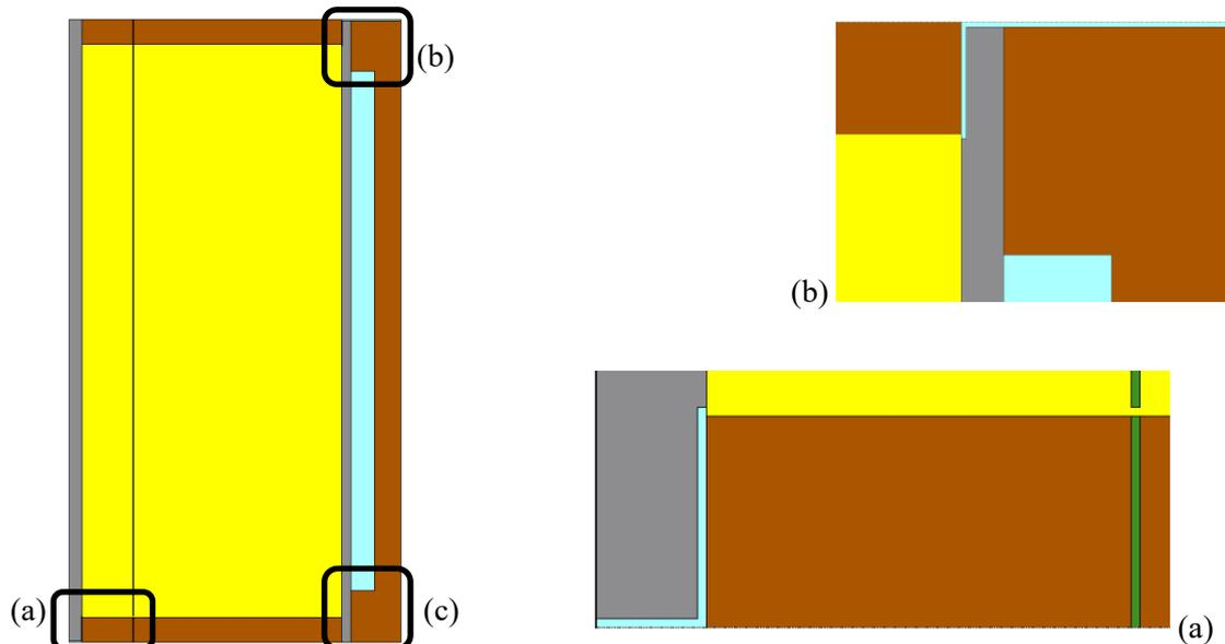
**Figure 1.** Left: The reference wall structure from top (indoors on the left). Right-bottom (a): L-shaped geometry of the inlet air gap. Right-top (b): L-shaped geometry of the outlet air gap at the adjacent wall stud. The outlet gap next to the inlet gap (c) was symmetrical to the adjacent stud outlet gap (b). The zoom level varies.
