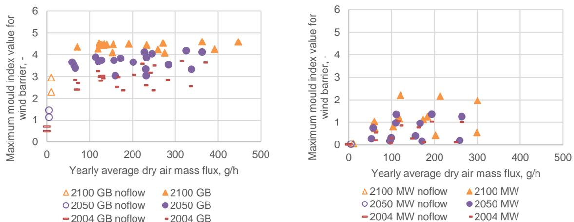
**Figure 2.** The maximum mould index value in the interior surface of the gypsum board (GB) wind barrier as a function of the dry air mass flux through the structure without (left) or with (right) additional thermal insulation (MW). The left-most values are given a small horizontal displacement to show them better.
